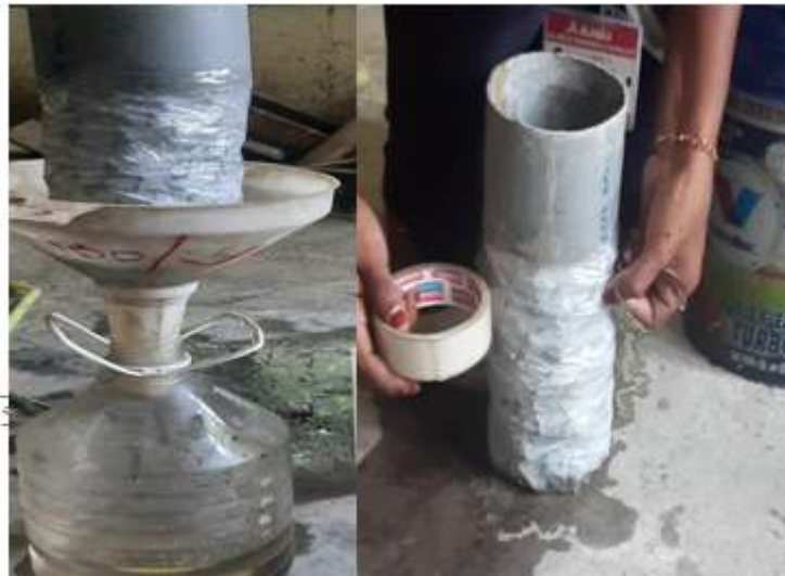
Fig 2. Permeability Testing Setup
